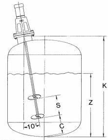
OFF CENTER MOUNTING FOR NON BAFFLED TANKS
